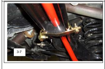
(2) Place outside edge of clamps at this point on the beam axle. (Fig. 3-5)
