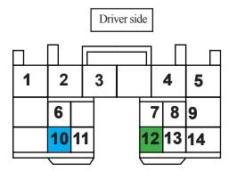
Positive +, Blue wire, pin 10 on connector. Negative -,Green wire, pin 12 on connector.
