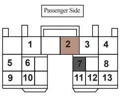
Positive +, Brown wire, pin 2 on Connector. Negative -, Gray wire, pin 7 on Connector.
