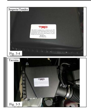
(f) Apply the TRD air filter warning label to the pre-cleaned area (Sequoia/Tundra Fig. 3-4, Tacoma Fig. 3-5).
