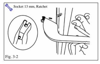
(b) Engage slot of center bracket under head of M8 x 25 bolt, slide upwards and snug with socket wrench to secure position. (Fig. 3-2)
