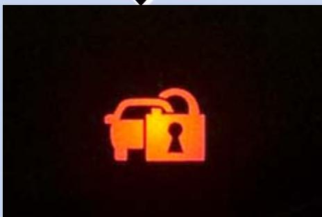
Security LED Turns ON solid for 30 Seconds
