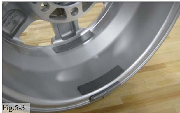
**STOP** NOTE: Make sure that the tire bead and tool does not interfere with the main body of the sensor and the bead does not clamp the sensor.
