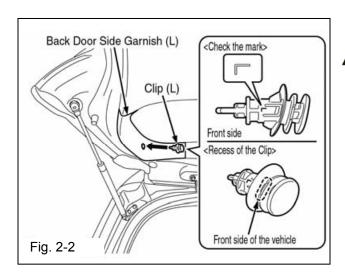
**NOTE:** For left hand clip the (L) mark and the recess faces the front of the vehicle.
