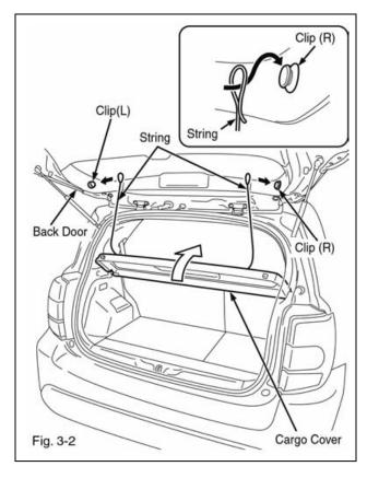
(b) Hook the pieces of string from the cargo cover to the clips (R and L) of the backdoor. (Fig. 3-2)
