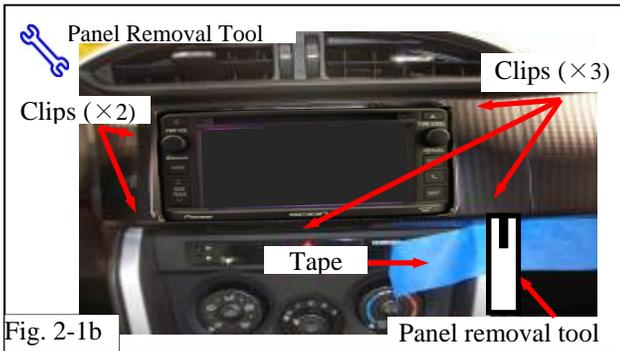
**DIO Disassembly (\*If Base DA pre-installed)**
